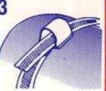
Feed other end of banding around objects to be clamped and through slot in housing
